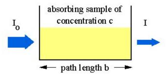
Modern absorption instruments can usually display the data as either transmittance, %-transmittance, or absorbance. An unknown concentration of an analyte can be determined by measuring the amount of light that a sample absorbs and applying Beer's law. If the absorptivity coefficient is not known, the unknown concentration can be determined using a <u>working curve</u> of absorbance versus concentration derived from <u>standards</u>.
